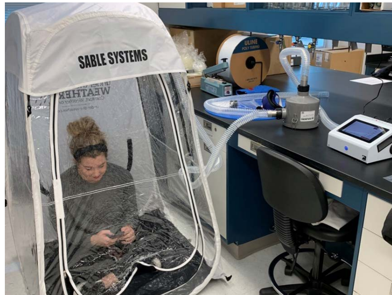
Craig Porter, Ph.D., used a portion of his Team Science Voucher Award to purchase the latest portable devices to more quickly measure energy expenditure of burn patients, which can be used to determine a patient's food/nutrient needs.
